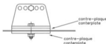
The minimum area of contact between bodyshell /chassis and counter plate is 40cm<sup>2</sup> for each fixing point. Any movable ballast system is forbidden.
